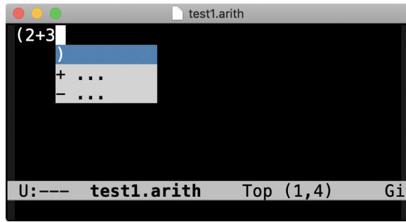
Figure 2. A screen shot of the three simple candidates popped up for the program text '(2+3' in an arithmetic language
